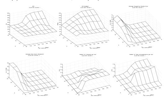
FIG. 5: TCP performance as the function of the buffer size *S*, in the piconet with two slaves. ((a) Round-trip time (RTT). (b) Goodput. (c) Mean size of the congestion window. (d) Mean value of the slow start threshold. (e) Time-out rate. (f) Fast retransmission rate.)
