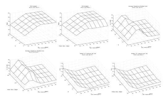
FIG. 9: TCP performance in the piconet with seven slaves. ( (a) Goodput as the function of the scheduling parameter M. (b) Goodput as the function of token rate. (c) Mean size of the congestion window as the function of the scheduling parameter M. (d) Mean size of the congestion window as the function of token rate. (e) Time-out rate as the function of the scheduling parameter M.(f) Time-out rate as the function of token-rate.)
