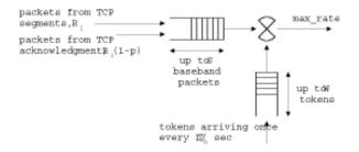
FIG. 10: Queueing model of the token bucket with finite capacity, accepting two types of packets.
