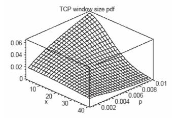
FIG. 3: Probability density function of TCP window size versus window size and segment loss probability.
