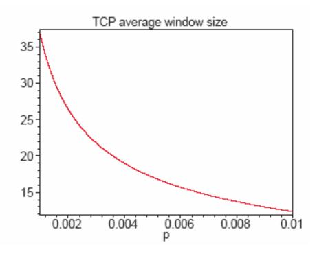
FIG. 4: Mean value of the TCP window size versus the segment loss probability.
