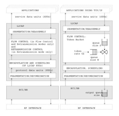
FIG. 1: Architectural blocks of the Bluetooth L2CAP layer (control paths not shown for clarity)((a) Original specification from<sup>9</sup>. (b) Implementation of the Flow Control mode.).
