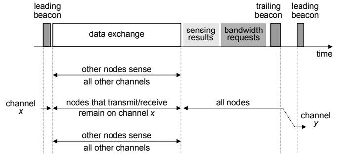
Fig. 1. Superframe format: some nodes transmit and receive data, some have just finished transmitting and undertake sensing, some have been sensing and report back to the CPAN coordinator.
