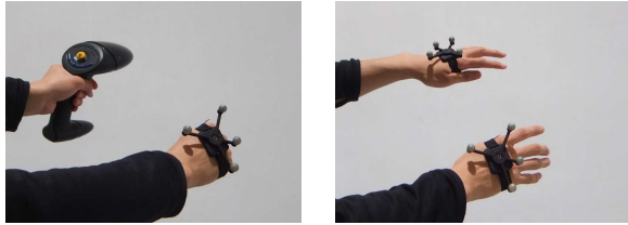
(a) Hand and wand (b) 2 hands Figure 3: Input devices for gesture interaction.
